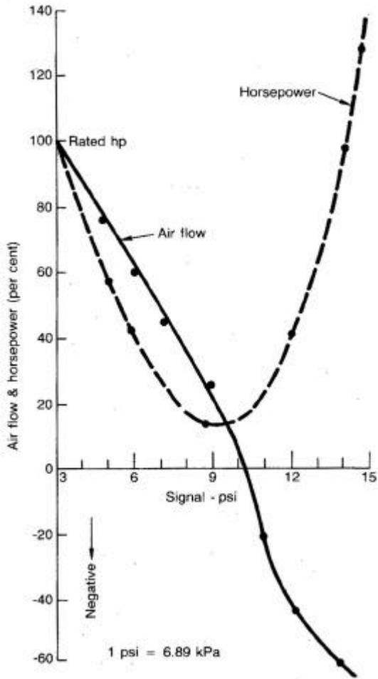
Figure 5 Air Flow and Horsepower Vs. Signal
