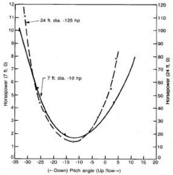
Figure 6 Horsepower Vs. Pitch Angle
