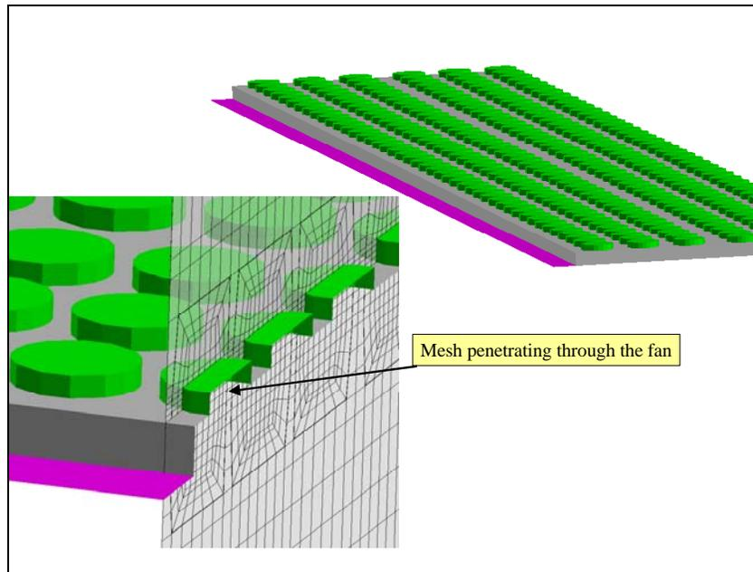
Figure 6: Fan model with mesh through the fan body
