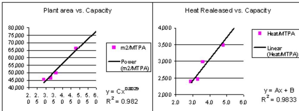
**Figure 2. Plant area and heat release versus capacity [2]**
