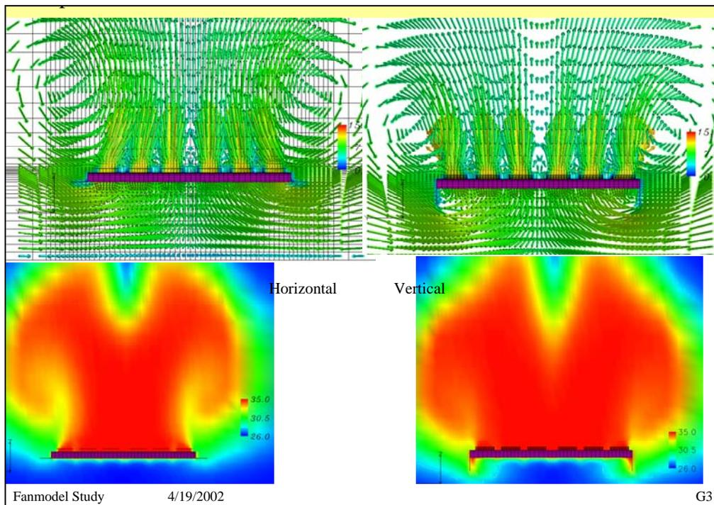
**Figure 7: Comparison of 10 ft. horizontal & vertical skirts, parallel wind**
