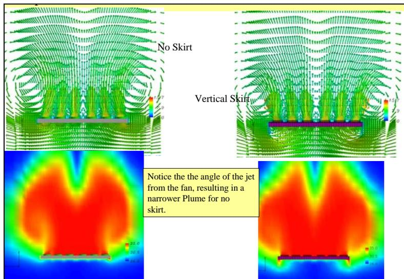
Figure 10: Comparison of no-skirt and vertical skirt, parallel wind case.
