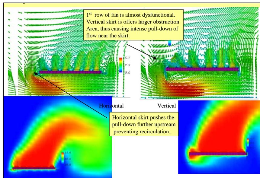
**Figure 8: Comparison of 10ft horizontal and vertical skirts, crosswind case.**
