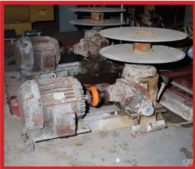
*Typical motor, shaft and gearbox fan drive.*
