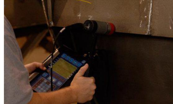
Testing structural natural frequency set on displacement
