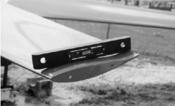
Mount Protractor on Flat bar as base and place it approximately 1" from tip of blade.
