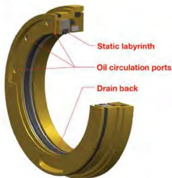
seal vendors claim that their internal O-ring design will move or adjust to block the leak path when the seal is not rotating. This O-ring concept has proven to be ineffective in the past (“Pump Zone” by Heinz Bloch). I’ve consulted with Bloch for years and agree that the inner O-ring does not work as designed. Even if the O-ring worked, a gearbox seal needs to retain oil in a dynamic flooded condition as well as static.
