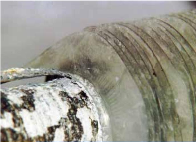
**FIG. 6** Water spray loosens the L-wrap type of fin.
