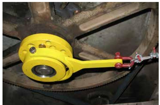
FIG. 10 DG-II anti-rotation device
