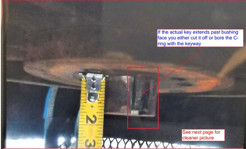
With this style Taper-lock bushing you must use the universal spacer that comes in the kit as per instructions if you plan to mount directly to the pulley bushing. But as you have a shaft extended down (past bushing face) you have a few options.
