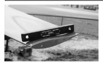
Mount Protractor on Flat bar as base and place it approximately 1" from tip of blade.
