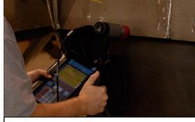
Testing structural natural frequency set on displacement
