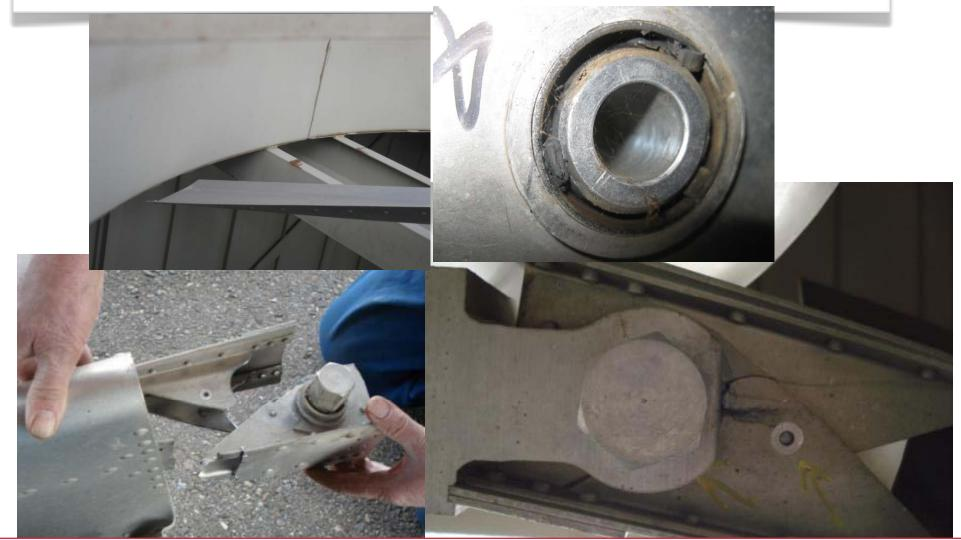
Moore fan blades depend on a rubber bushing at the connection, rubber ages so these need to be replaced when they get hard. Typically, everyone over pitches these fans in the field based off using amp draw to set max pitch. This is a very poor practice, which overloads these rubber joints, which creates a fan blade failure as you see here.
