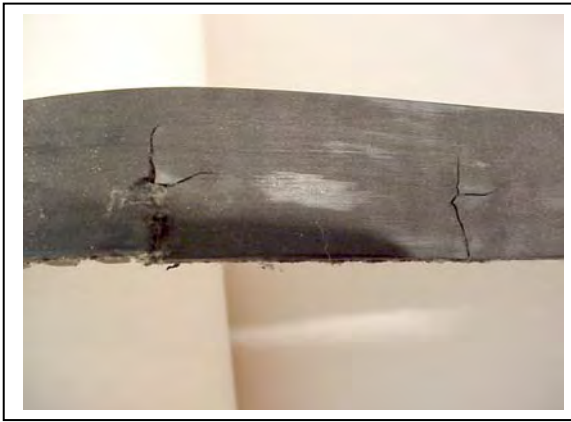
Figure 4 – Tensile Cord Failure From Debris
