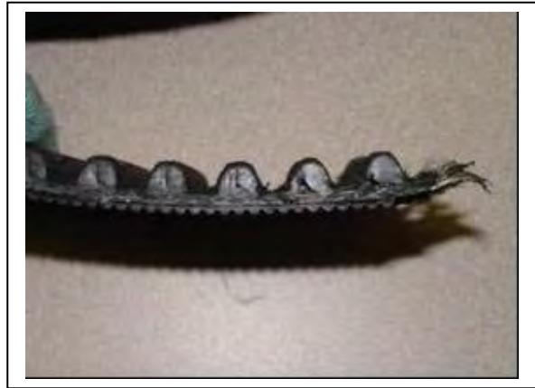
Figure 5 - Shock loaded Tooth Failure
