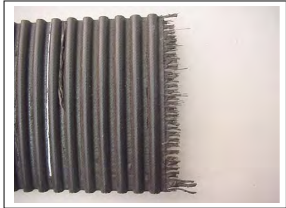
Figure 5 – Tensile Cord Crimp Failure
