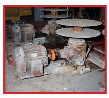
Typical motor, shaft and gearbox fan drive.
