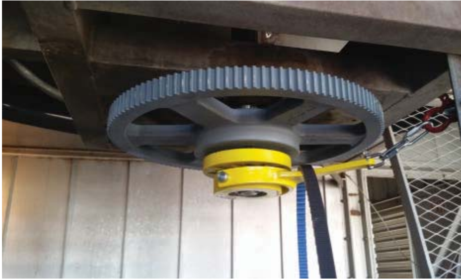
This ARD, bolted onto an existing fan pulley bushing, gets maximum efficiency at the gas plant where it is installed.
