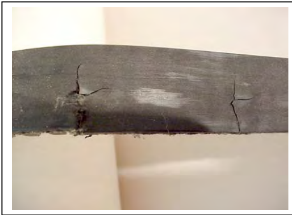
Figure 4 – Tensile Cord Failure From Debris
