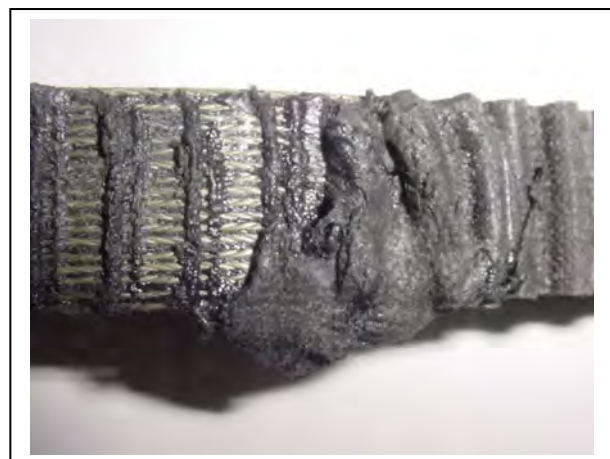
Figure 3 - Poly Chain GT2 Failure Due To Excessive Heat
