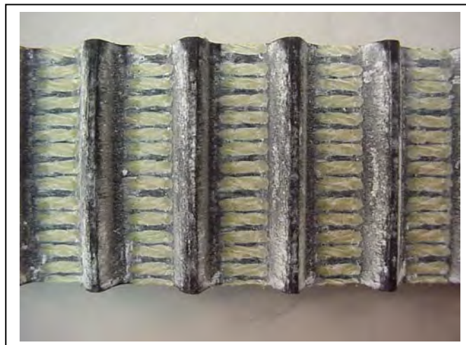
Figure 1- Belt Wear From Abrasive Atmosphere
