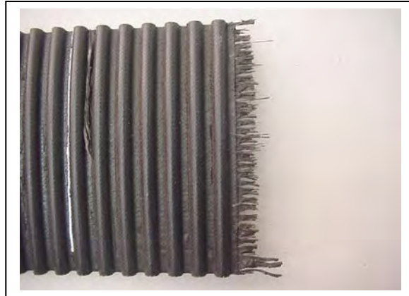
Figure 5 – Tensile Cord Crimp Failure
