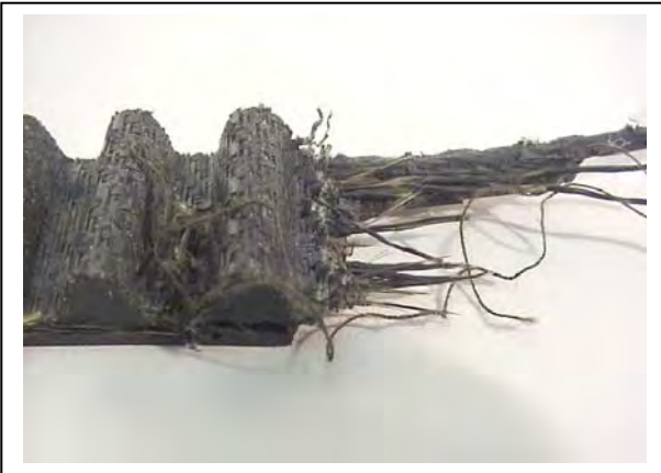
Figure 4 - Shock load Failure
