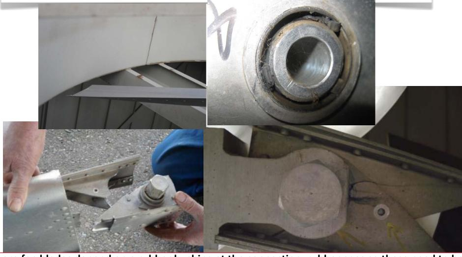
Moore fan blades depend on a rubber bushing at the connection, rubber ages so these need to be replaced when they get hard. Typically, everyone over pitches these fans in the field based off using amp draw to set max pitch. This is a very poor practice, which overloads these rubber joints, which creates a premature fan blade failure as you see here.
