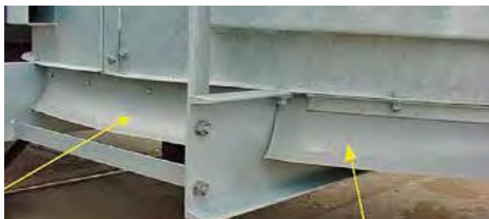
FIG. 4 An inlet bell can be part of a fan ring or added later.
