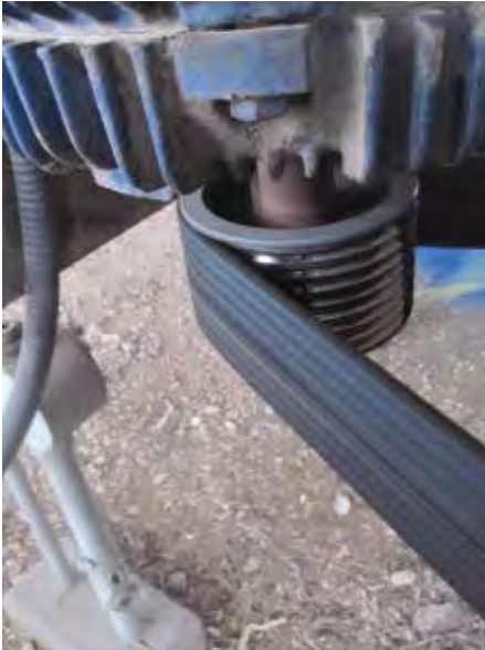
The lack of belt wrap and the shin on the pulley from belt slip shows why V-belts are not very effective for driving air coolers.
