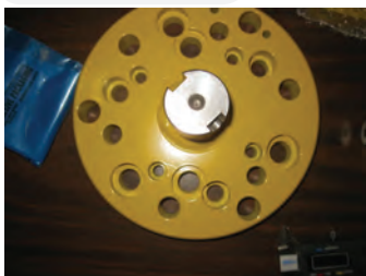
Figure 1: Flange plate c/w stub shaft
