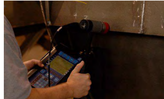
Testing structural natural frequency set on displacement
