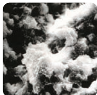
Millions of micro-pores retain the oil in Solid Oil.
