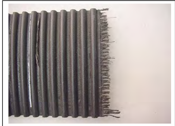
Figure 5 – Tensile Cord Crimp Failure
