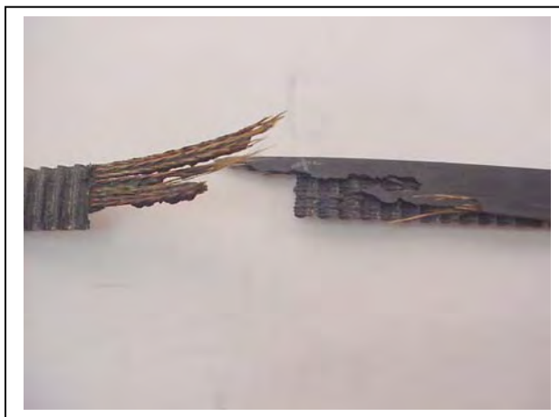
Figure 1 - Normal Tensile Failure
