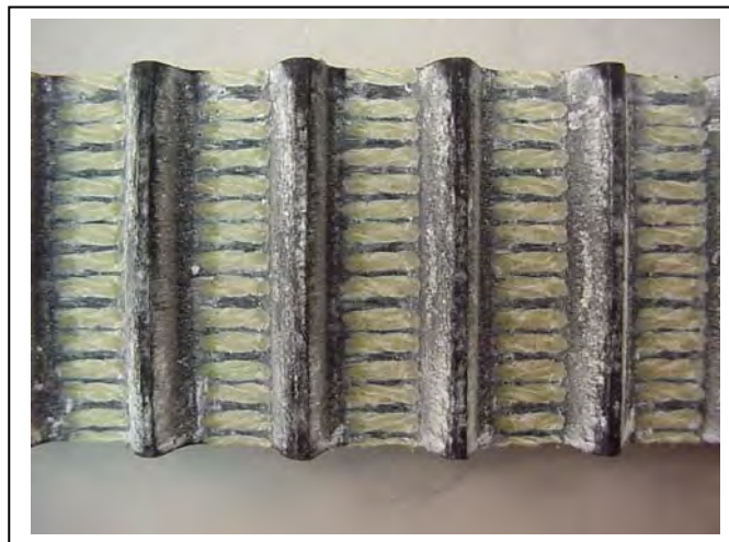
Figure 1- Belt Wear From Abrasive Atmosphere
