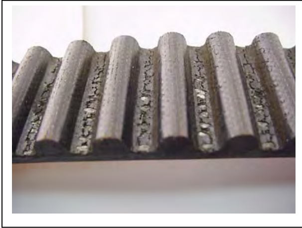
Figure 4 - Sub-minimal Sprocket Belt Failure
